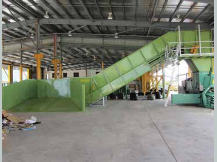
Above ground with 5 metre heavy duty ramp and horizontal feed section. 1800mm wide live feed area, 30,000LB chain, 28deg incline with curved head section complete with access ladder, service platform and head conveyor access.
