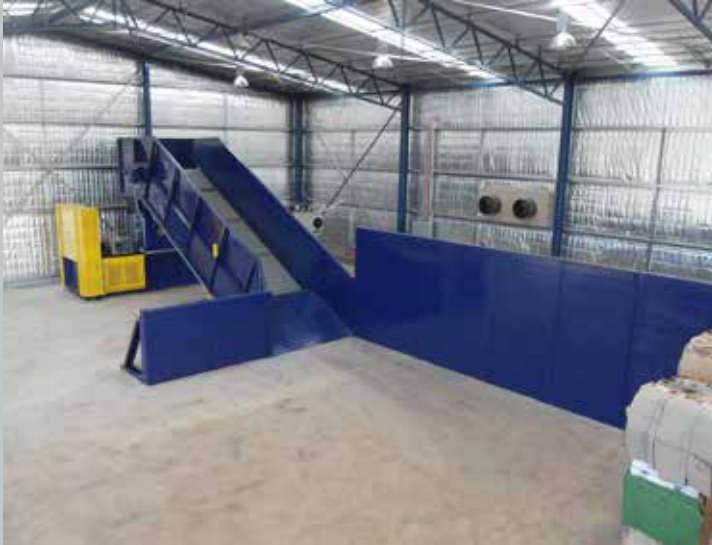
Above ground end push conveyor with heavy duty inclined ramp. 1500mm wide live feed area, 15,000LB chain, 28deg incline with straight head. Prefabricated bolted sectional push walls 1500mm and 2400mm high.
